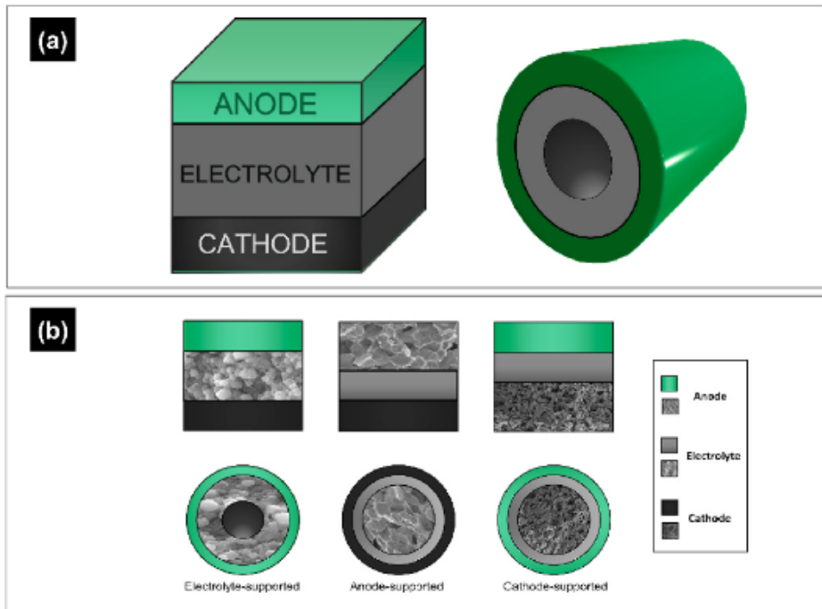
Fig. 2. SOFC geometries: (a) 3D model of the planar and tubular cell, (b) cross-sections of electrolyte-, anode-, and cathode-supported cells for both planar and tubular geometry.
