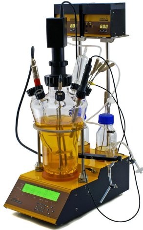
© MINIFOR laboratory fermentor-bioreactor advanced kit 1L vessel-right" by LambdaCZ
