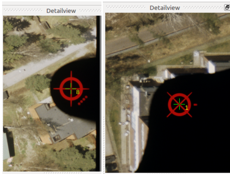
FIGURE 7.6. Fiducial marks in the Detailview at 8× magnification: left an edge mark, right a corner mark.
