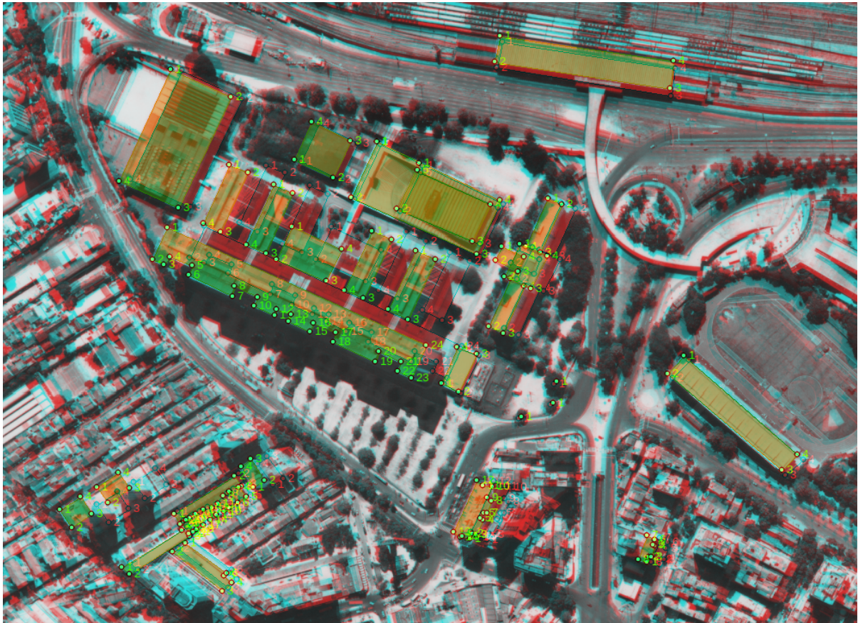
FIGURE 10.9. A bigger sample of stereo plotter production showing several urban features in the Rio area.
