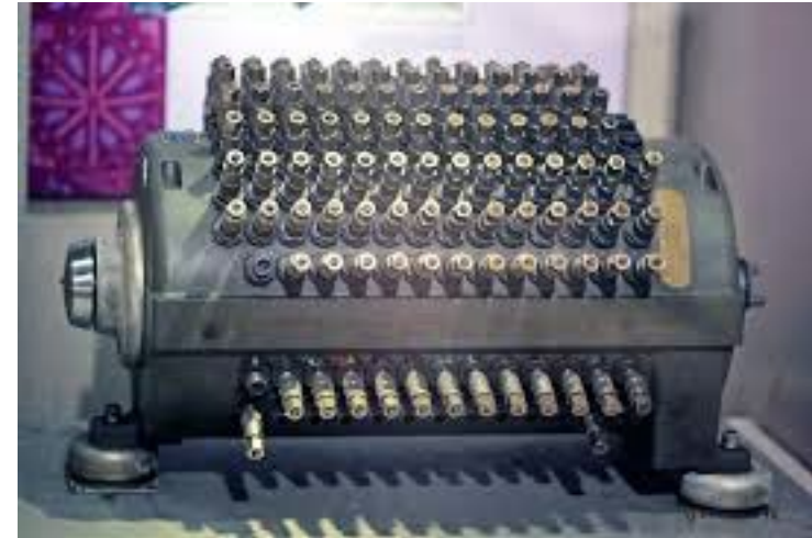
Memory drum of ILLIAC I, on display at the Spurlock Museum . Image by Wikipedia user Rama. Image is available under CC BY-SA 2.0 Fr .
