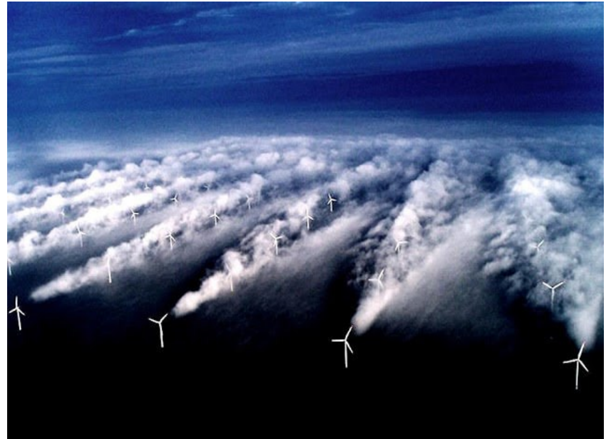
Wake interactions in Horns Rev Offshore Wind Farm, Denmark. (Photo by Christian Steiness / Vattenfall)
