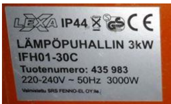
Specification plate of an electrical heater.
