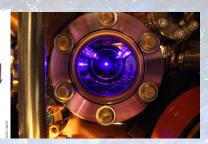
The technological novelty with optical lattice clocks is, that the wavelength used is *in the optical range* and not in the microwave range, like for more traditional atomic clocks. The more rapid oscillations allow for more precise time keeping.
