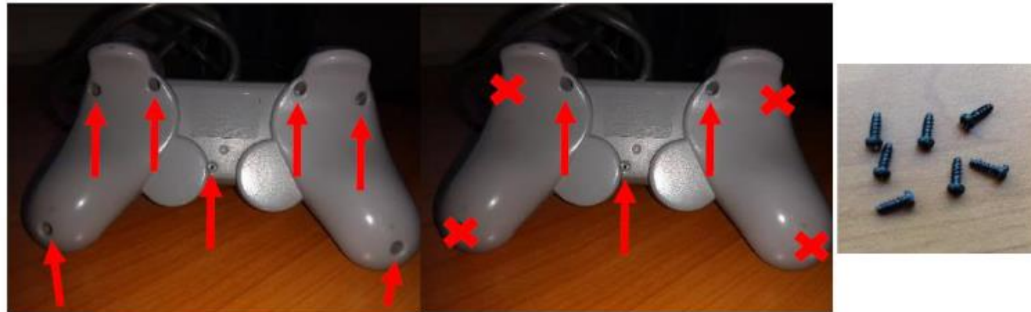
Figure 2 and 3. Difference between the screws in original (left) and improved (middle). Picture of screws on the right.
