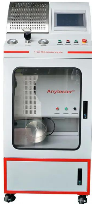
PICTURE: Lab Scale Melt Spinning Machine
